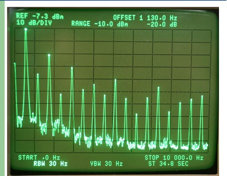
Pro III driven into clipping to meet the 2 W. into 8 ohm spec.
