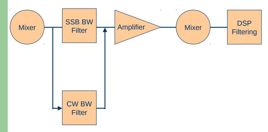
This keeps the undesired strong signals from progressing down stream to the next stages.
