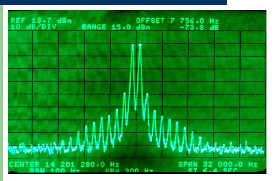
Note: Must add 6 dB to spectrum analyzer IMD measurements to compare to League & OEMs.
