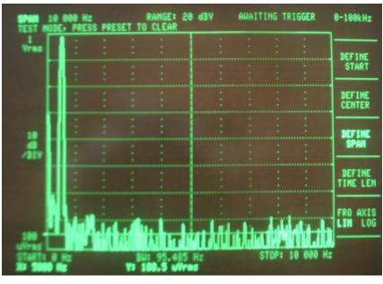
A single 500 Hz "dit" with 3<sup>rd</sup>, 5<sup>th</sup>, 7<sup>th</sup> & 9<sup>th</sup> harmonics to 4.5 kHz.
